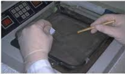
Taking the floating sections onto slide
