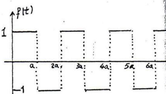
$$\begin{aligned} L\{f(t)\} &= L\{U(t)\} - 2 \sum_{n=1}^{\infty} (-1)^{n+1} L\{U(t-na)\} = \\ &= \frac{1}{s} - 2 \sum_{n=1}^{\infty} (-1)^{n+1} \frac{e^{-nas}}{s} = \frac{1}{s} - \frac{2e^{-as}}{s(1+e^{-as})} = \\ &= \frac{1 - e^{-as}}{s(1+e^{-as})} = \frac{e^{1/2as} - e^{-1/2as}}{s(e^{1/2as} + e^{-1/2as})} = \frac{1}{s} \tanh\left(\frac{1}{2}as\right). \end{aligned}$$
