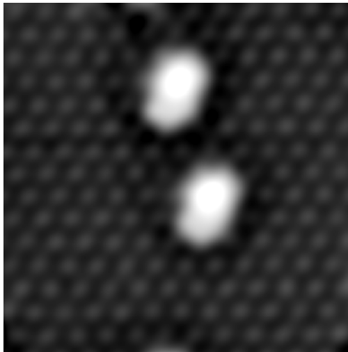
Figure 1-19. 5 nm \times 5 nm area of a hydrogen-passivated Si (111) surface, imaged in an STM with a tip potential of -1.5 V. The subtle hexagonal structure represents H-covered Si atoms, while the two prominent white patches arise from dangling bonds where the H atoms have been removed (these appear non-circular because of the somewhat irregularly shaped tip). Courtesy of Jason Pitters and Bob Wolkow, National Institute of Nanotechnology, Canada.
