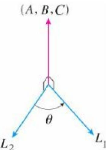
$$(A, B, C) = (a_1, b_1, c_1) \times (a_2, b_2, c_2) = \begin{vmatrix} i & j & k \\ a_1 & b_1 & c_1 \\ a_2 & b_2 & c_2 \end{vmatrix}$$
