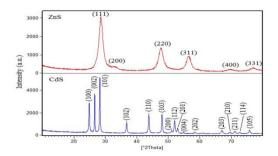
It is worth mentioning that the XRD patterns can clarify the nanosize nature of a substance. Sharp lines or peaks indicate large or perfect crystals while small crystallite size materials are characterized by broad peak. The absence of peaks from the XRD pattern characterize amorphous samples.
