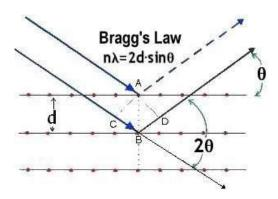
X-ray diffraction (XRD) is used for the identification of different phases of crystalline compounds and useful information can be obtained from the diffraction pattern (like the crystallite size, d spacing, miller indices, micro strain etc.).
