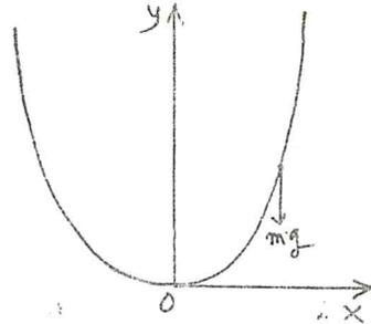
$$\therefore d\underline{r} = dx \underline{i} + 2ax dx \underline{j}, dW = -2mgax dx$$
