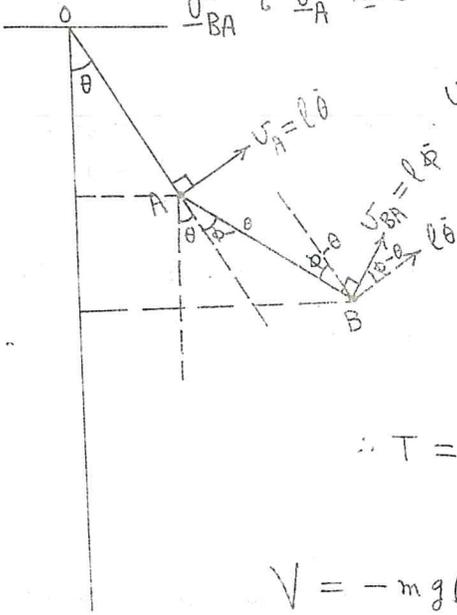
$$v_B^2 = l^2 \dot{\theta}^2 + l^2 \dot{\phi}^2 + 2l^2 \dot{\theta} \dot{\phi} \cos(\phi - \theta)$$
