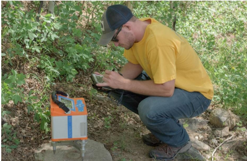
Figure 1: The measurement of the gravity data by a gravity meter during a survey.
