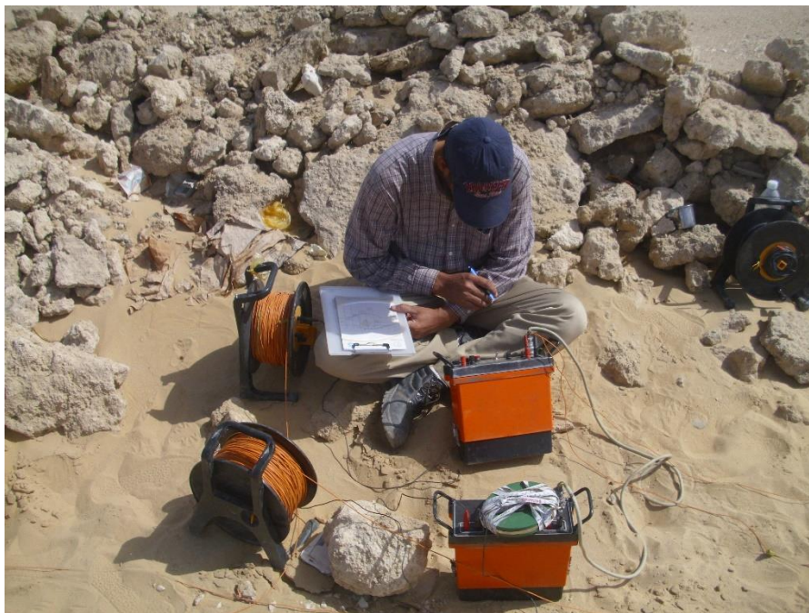
Figure 12: Recording the electric resistivity data on the field sheet.
