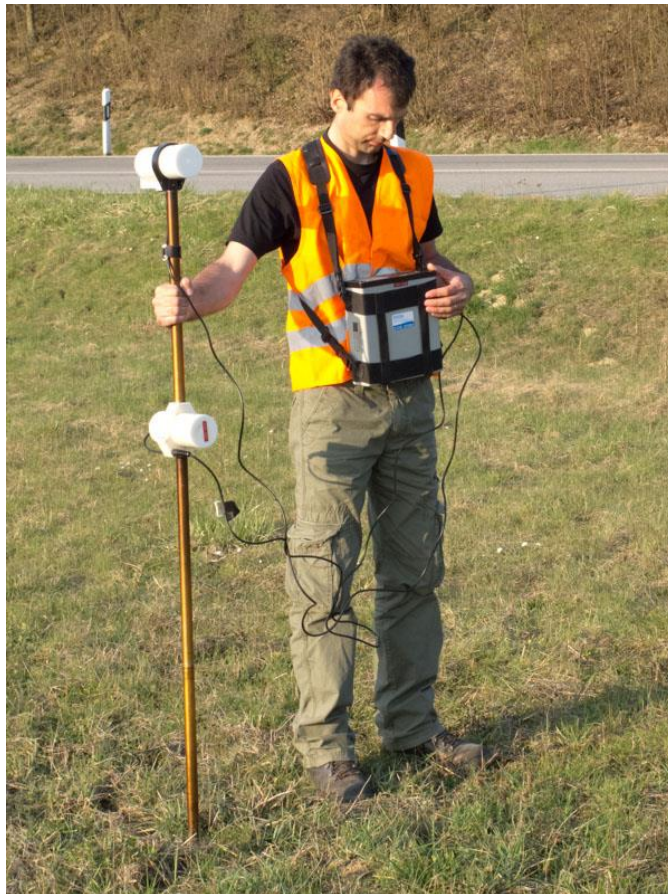
Figure 4: A magnetic survey where a magnetometer is used to detect the magnetic anomalies caused by buried steel objects.
