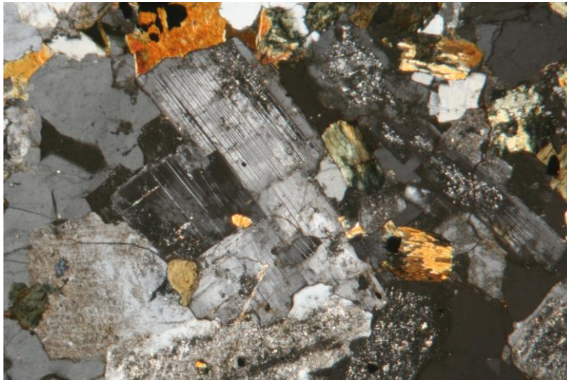
Plagioclase, quartz, alkali-feldspars, and biotite in a granodiorite. XPL image, 2x (Field of view = 7mm)
