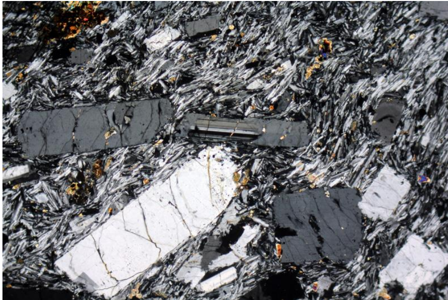
Sanidine and plagioclase in trachyte. XPL image, 10x (Field of view = 2mm)
