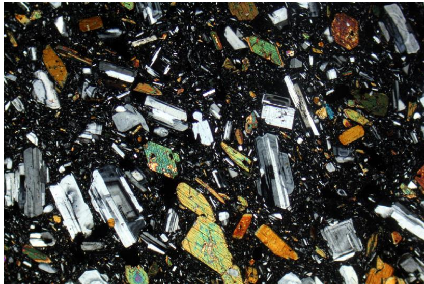
Hornblende and plagioclase crystals in a Andesite. XPL image, 2x (Field of view = 7mm)
