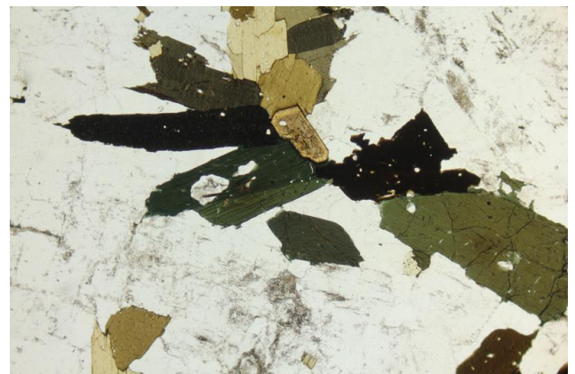
Hornblende (green) and biotite (brown) crystals in granite. PPL image , 2x (Field of view = 7mm)
