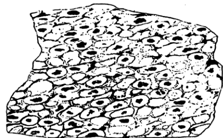
Orbicular texture consisting of chromite nuclei "dark" surrounded by sheath of olivine "light".
