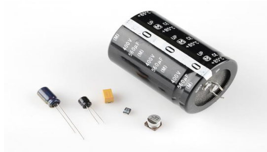
An assortment of through-hole and surface-mount electrolytic capacitors. Notice each has some method for marking the cathode (negative lead).
