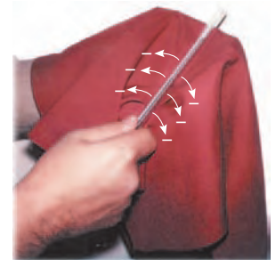
Figure 1.2 When a glass rod is rubbed with silk, electrons are transferred from the glass to the silk. Because of conservation of charge, each electron adds negative charge to the silk and an equal positive charge is left behind on the rod. Also, because the charges are transferred in discrete bundles, the charges on the two objects are \pm e , or \pm 2e , or \pm 3e , and so on.
