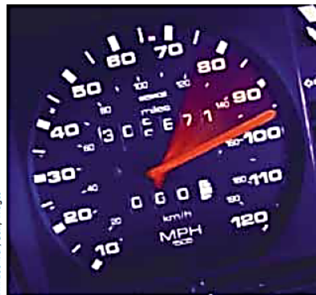
Figure 1.3 The speedometer of a vehicle that shows speeds in both miles per hour and kilometers per hour.
