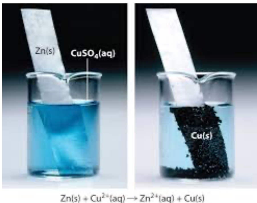
Figure 1: Dissolving of Zn and Dissolving of \text{Cu}^{+2}
