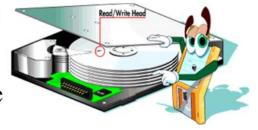
heads, damage to the surface of the disk, or all three. This is usually called a *head crash*, two of the most frightening words to any computer user. :^) The most common causes of head crashes are contamination getting stuck in the thin gap between the head and the disk, and shock applied to the hard disk while it is in operation.
