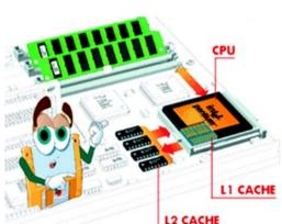
2) External cache (L2) resides on the motherboard. The L2 cache is an area of high-speed memory that improves performance by reducing the average memory access time. L2 cache is also called SRAM.
