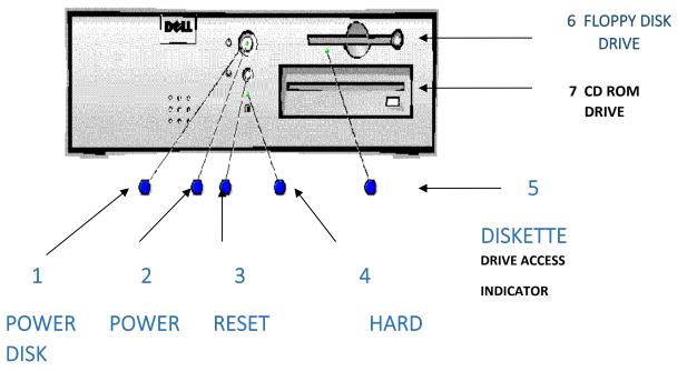
The computer is a machine that processes data according to a set of instructions that are stored internally either temporarily or permanently. The computer has either external or internal peripherals attached to it. The picture below displays two internal devices—the floppy disk drive and CD ROM drive.
