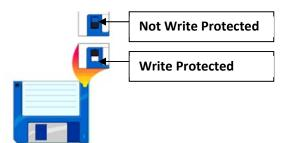
Every disk comes with a write-protect tab. The tab provides protection against erasing or replacing information on a floppy disk. You can
