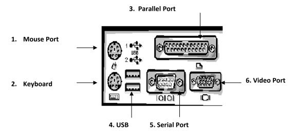
computer. Included are pictures of the cable connectors for different peripherals attached to the computer.
