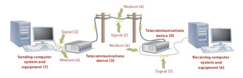
Figure shows a general model of telecommunications. The model starts with a sending unit (1) such as a person, a computer system, a terminal, or another device that originates the message. The
