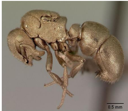
Sputter-coated ant specimen ( Aulacopone relictica ) for SEM examination).
