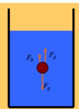
Weight of the ball force of pushing on the ball + Stocks force.
