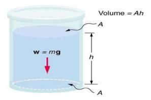
Pressure is the weight of the fluid *mg* divided by the area *A* supporting it (the area of the bottom of the
