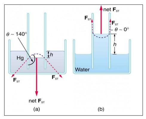
A simple relationship determines how far the water is pulled up the tube (see Figure 5). The force upwards due to the surface tension is given by the following
