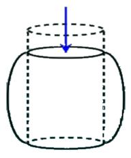
Compressive stress results in deformation which shortens the object but also expands it outwards.
