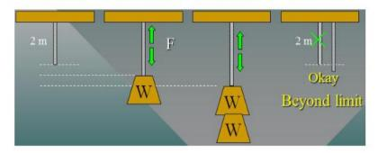
If the stress exceeds the elastic limit, the final length will be longer than the original  $2\ m.$
