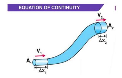
Now, consider the fluid flows for a short interval of time in the tube. So, assume that short interval of time as  $\Delta t$ . In this time, the fluid will cover a distance of  $\Delta x_1$  with a velocity  $v_1$  at the lower end of the pipe.
