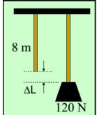
$$Y = 8.96 \times 10^{11} \text{ Pa; } F = 120 \text{ N; } L = 8 \text{ m; } A = 1.77 \times 10^{-6} \text{ m}^2; F = 120 \text{ N; } \Delta L = ???$$
