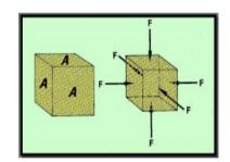
a bulk modulus B of elasticity.
