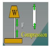
Strain is the relative change in the dimensions or shape of a body as the result of an applied stress:
