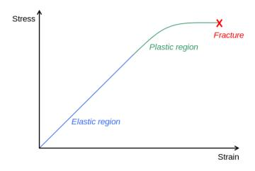
Diagram of a stress-strain curve, showing the relationship between stress (force applied) and strain (deformation) of a ductile metal.
