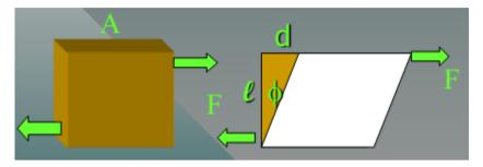
The shearing force F produces a shearing angle  $\varphi$ . The angle  $\varphi$  is the strain and the stress is given by F/A as before.
