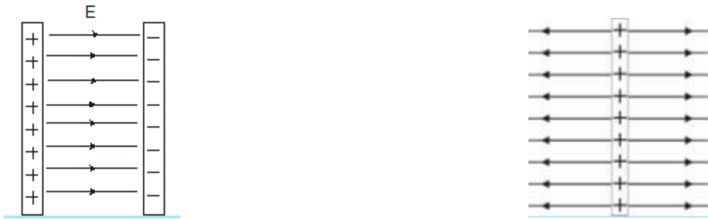
Electric field lines due two surface charge to +ve line Electric field lines due to +ve line
