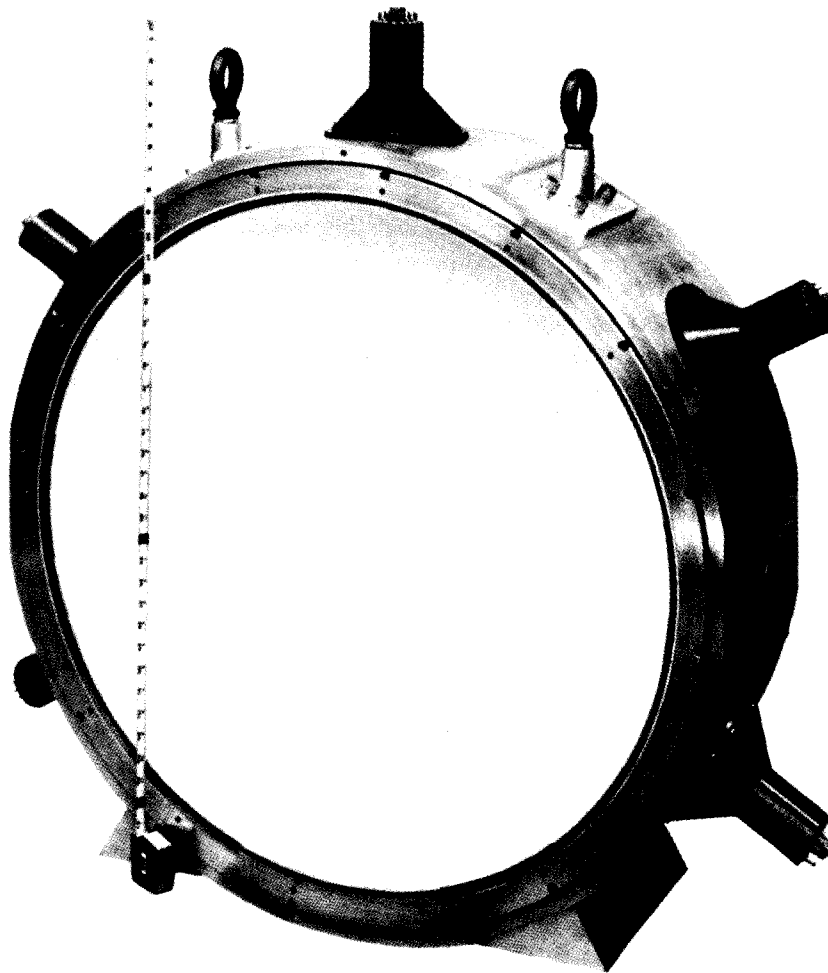
Figure 6.16 A special 30-in (0.762-m) diameter scintillator crystal coupled to six photomultiplier tubes (from Harshaw Chemical Company).
