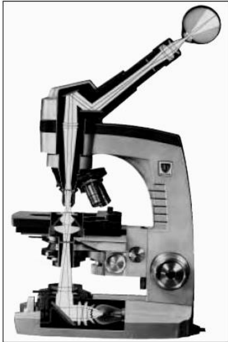
The light pathway of a microscope
