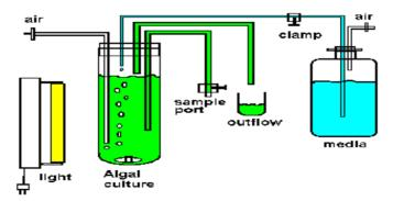
Air is also pumped into the culture vessel. This air passes down a long glass tube to the bottom of the culture and bubbles up. This serves to keep the culture well suspended as well as high in oxygen and CO2. The air flowing into the culture vessel flows out through an outflow tube. As fresh medium is added
