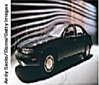
Figure 14.13 Laminar flow around an automobile in a test wind tunnel.
