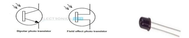
When light sensitive area is exposed to light then a small amount of current generates at base terminal and it causes to flow large current from collector to emitter. The photo transistors are available in both BJT and FET transistor types. These are named as photo-BJTs and photo-FETs.
