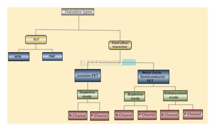
The transistors classification can be understood by observing the above tree diagram. Transistors are basically classified into two types; they are Bipolar Junction Transistors (BJT) and Field Effect Transistors (FET). The BJTs are again classified into NPN and PNP transistors. The FET transistors are classified into JFET and MOSFET.
