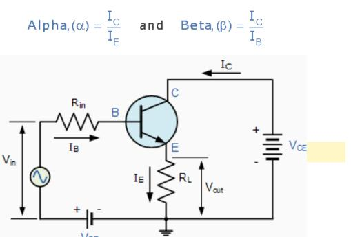
Where: " $I_C$ " is the current flowing into the collector terminal, " $I_B$ " is the current flowing into the base terminal and " $I_E$ " is the current flowing out of the emitter terminal.
