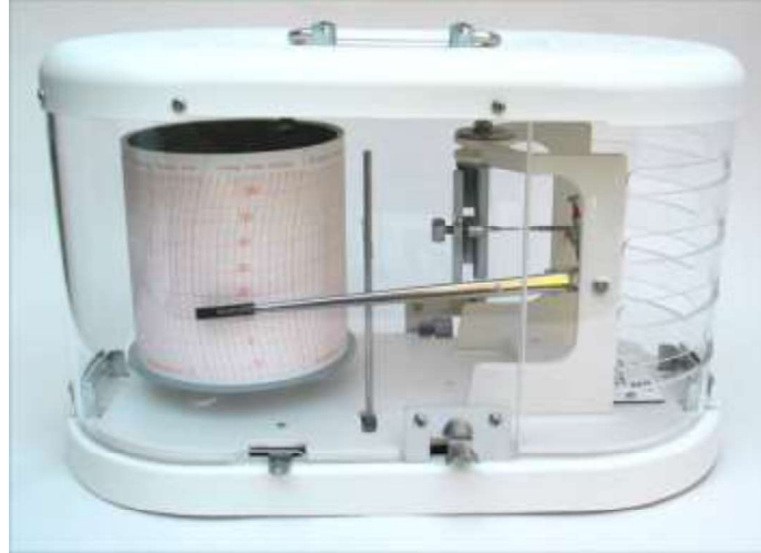
Figure 2.4: An actual thermograph
