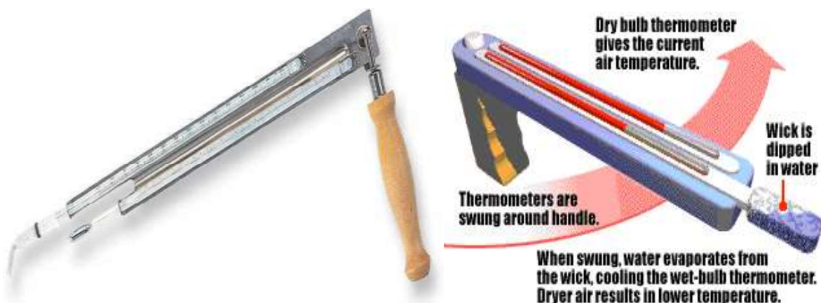
Figure 2.6: (Left) An actual sling psychrometer; (Right) A schematic of a sling psychrometer
