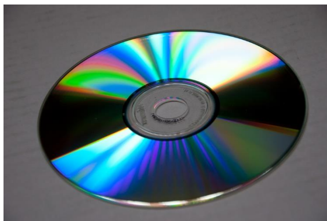
Figure: The colors reflected by this compact disc vary with angle and are not caused by pigments. Colors such as these are direct evidence of the wave character of light. (credit: Infopro, Wikimedia Commons)
