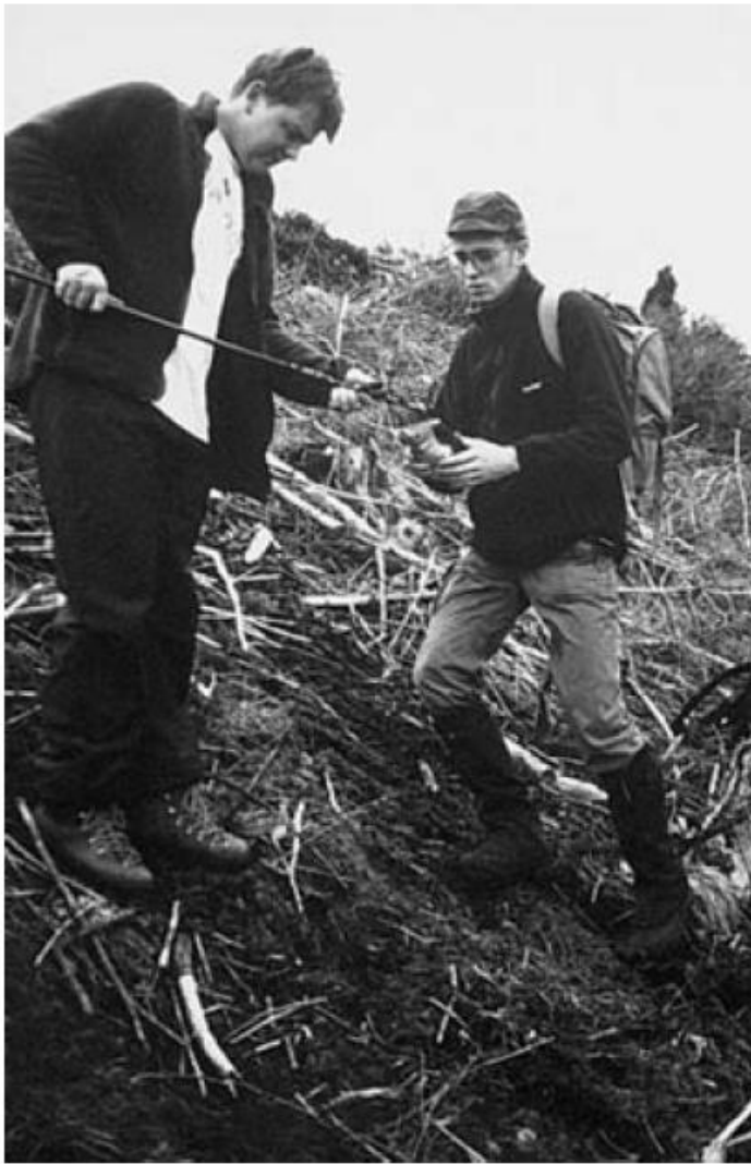
FIG. 8.13 Typical surface soil sampling in temperate terrains using hand augers over the Coed-y-Brenin copper prospect Wales
