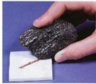
The red-brown streak of the mineral hematite
