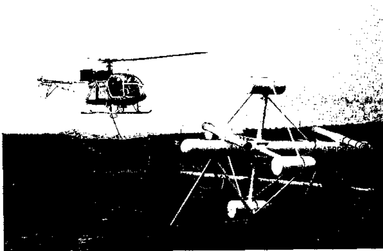
Figure 3.23 Eurocopter AS315 about to lift a 3-axis magnetic gradiometer system. Courtesy of Aerodat Inc., Canada
