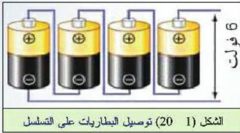
$$V_T = V_1 + V_2 + V_3 + \dots$$
