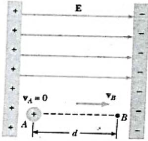
$$\Delta V = -Ed = -(8.0 \times 10^4 \text{ V/m})(0.50 \text{ m}) = -4.0 \times 10^4 \text{ V}$$
