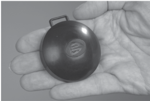
Figure 5.2 Passive radon detector. (Adapted with kind permission from Report HPA-RRP-001, Ionising Radiation Exposure of the UK Population: 2005 Review , by S. J. Watson et al., 2005, © Health Protection Agency.)
