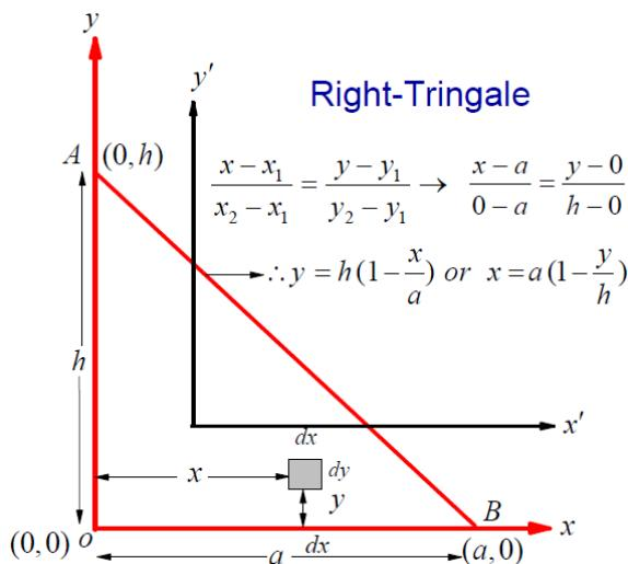
$$dm = \rho dx dy \rightarrow m = \rho \int_0^h \int_0^{a(1-\frac{y}{h})} dx dy = a \rho \left[ h - \frac{h^2}{2h} \right] = \frac{1}{2} a h \rho$$
