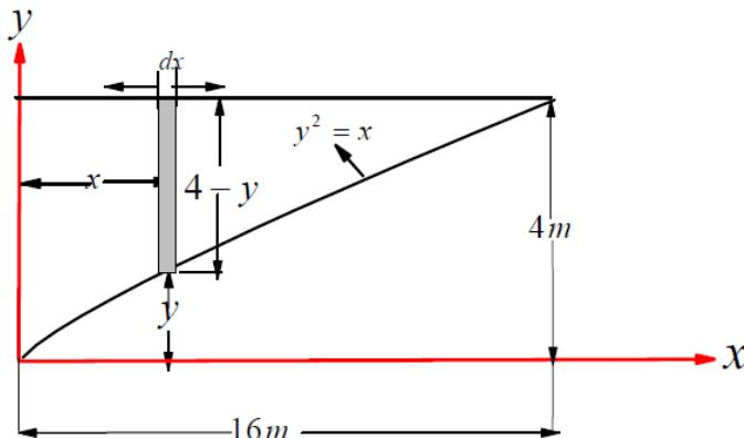
$$I_{yy} = \int x^2 dA = \int_0^{16} x^2 (4 - y) dx = \int_0^{16} x^2 \left( 4 - (x)^{1/2} \right) dx = \int_0^{16} \left( 4x^2 - (x)^{5/2} \right) dx = \frac{4(16)^3}{3} - \frac{2(16)^{7/2}}{7}$$
