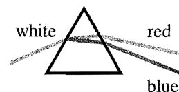
Fig. 2.10 Separation of white light into different colours by dispersion in a glass prism.
