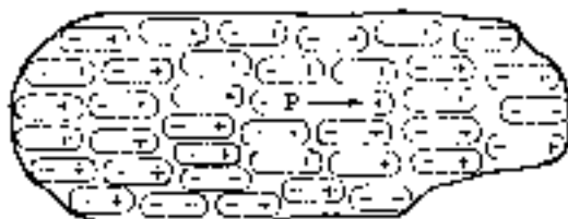
FIG. 4-1. A piece of polarized dielectric material. Each volume element is represented as a dipole \Delta p .
