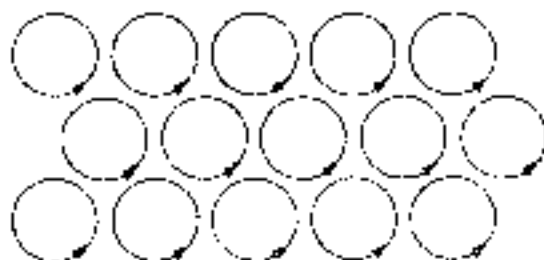
FIG. 10-1. Simplified picture of magnetic material consisting of atomic loop currents circulating in the same direction.
