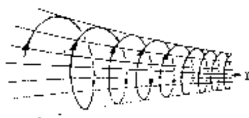
FIG. 14-1. The particle winds in a tighter and faster helix until it is reflected.
