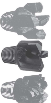
Figure 3-106: Drag bits with tungsten carbide inserts
