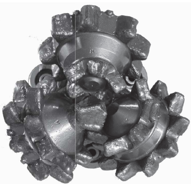
Figure 3-111: Soft formation roller bit
