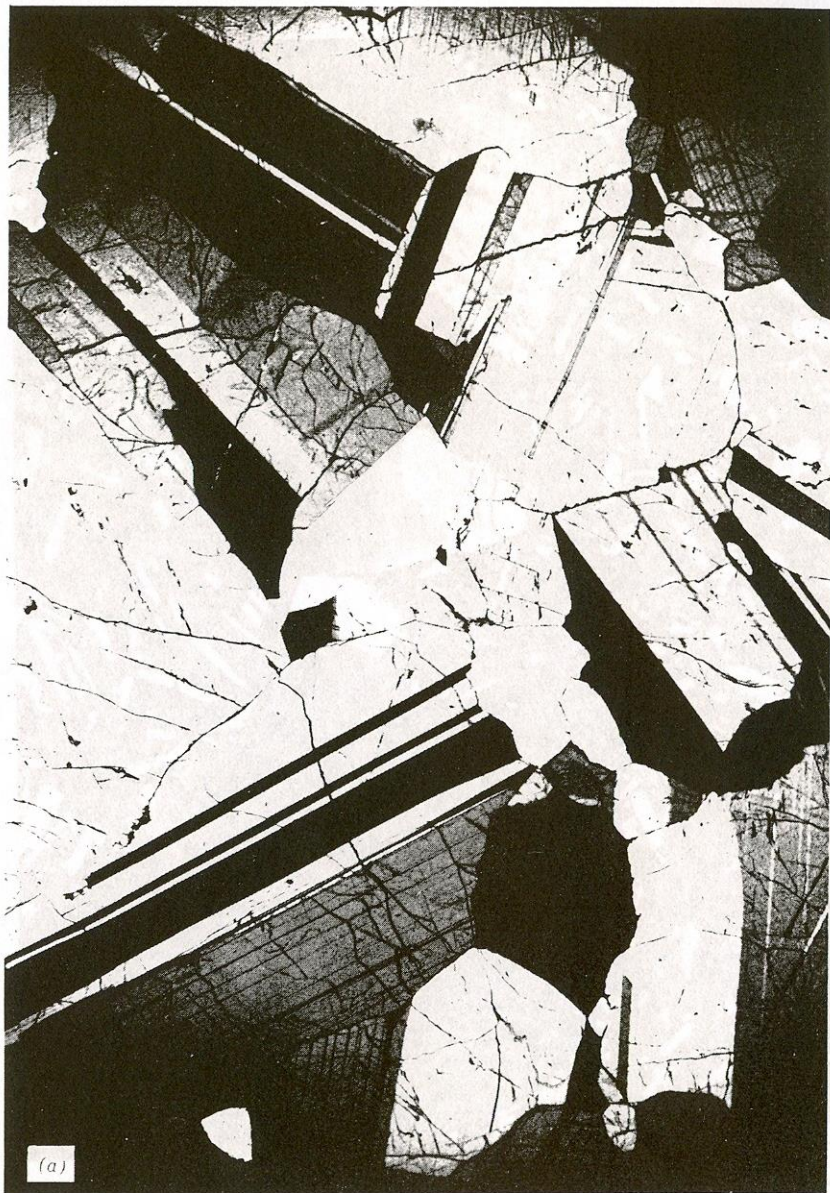
Figure 2.2 Photomicrographs of thin sections of fissured rocks, photographed in transmitted, polarized light (courtesy of H. R. Wenk). (a) Anorthosite with many intracrystalline and some intercrystalline fractures ( \times 6.5 ).
