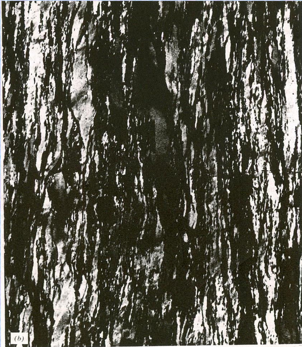
Figure 2.1 Photomicrographs of thin sections of rocks, viewed in polarized, transmitted light (courtesy of Professor H. R. Wenk). (b) Highly anisotropic fabric of a quartz mylonite ( \times 20 ).
