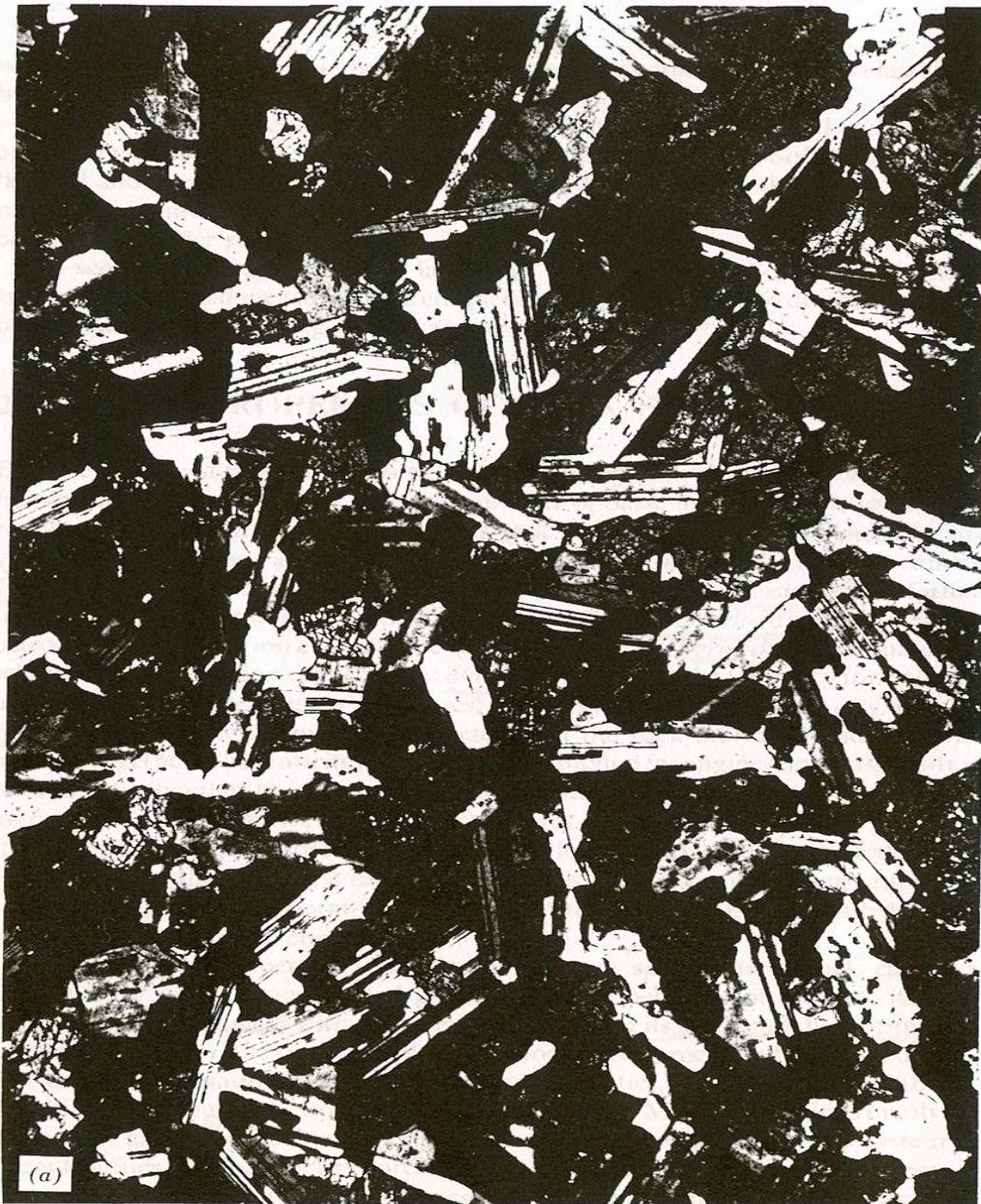
Figure 2.1 Photomicrographs of thin sections of rocks, viewed in polarized, transmitted light (courtesy of Professor H. R. Wenk). (a) Tightly interlocked fabric of a crystalline rock—diabase ( \times 27 ).
