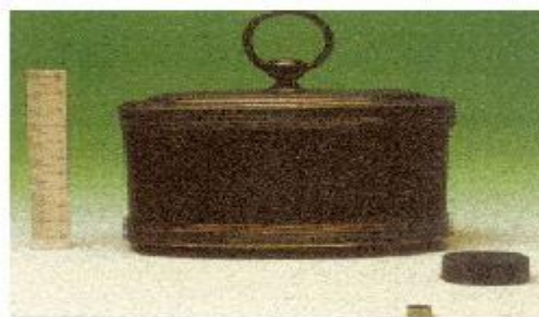
Figure 28 (b): Brass bound lodestone, ferrite block and NdFeB magnet: each store the same magnetic energy (~0.4J) & contain ~70% iron by weight, yet the mass has decreased a thousand-fold.
