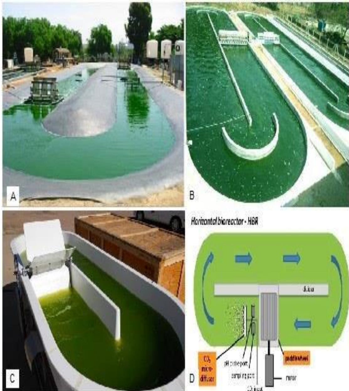
Fig: Open raceway ponds for algal cultivation, A. Raceway pond with thick dividing section (Source-SARDI, South Australia), B. Open raceway pond (Source-Arban Infrastructure Pvt. Ltd., Biotech division), C. Laboratory scale high rate algal pond (Source-New Mexico State University), D. Schematic of the horizontal pond or bioreactor (Source-Brown et al., 2015).
