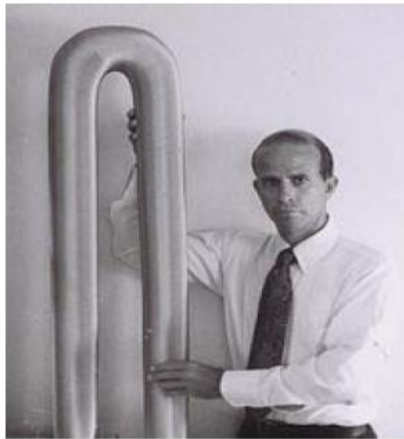
A rod of semiconductor-grade polysilicon. (Held by Leo Rogers of Polycrystalline Silicon Technology Corporation (P.S.T.)
