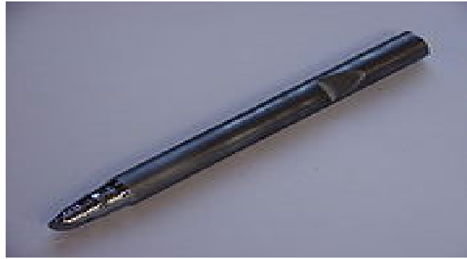
puller rod with seed crystal for growing single-crystal silicon by the Czochralski process
