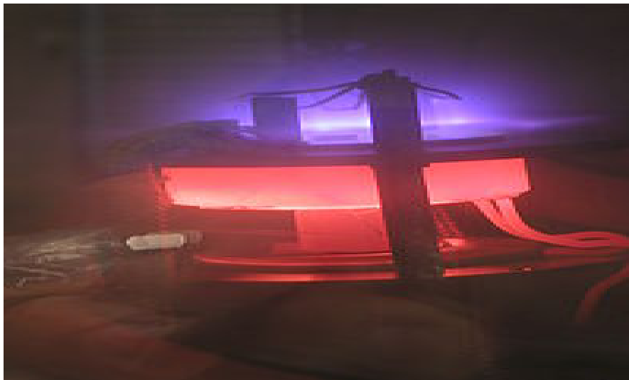
DC plasma (violet) enhances the growth of carbon nanotubes in this laboratory-scale PECVD apparatus.
