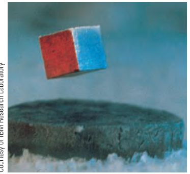
A small permanent magnet levitated above a disk of the superconductor YBa 2 Cu 3 O 7 , which is in liquid nitrogen at 77 K.
