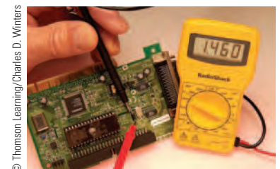
A digital multimeter is used to measure a voltage across a circuit element.
