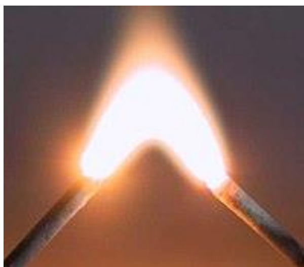
Figure (7): The Electric Arc
