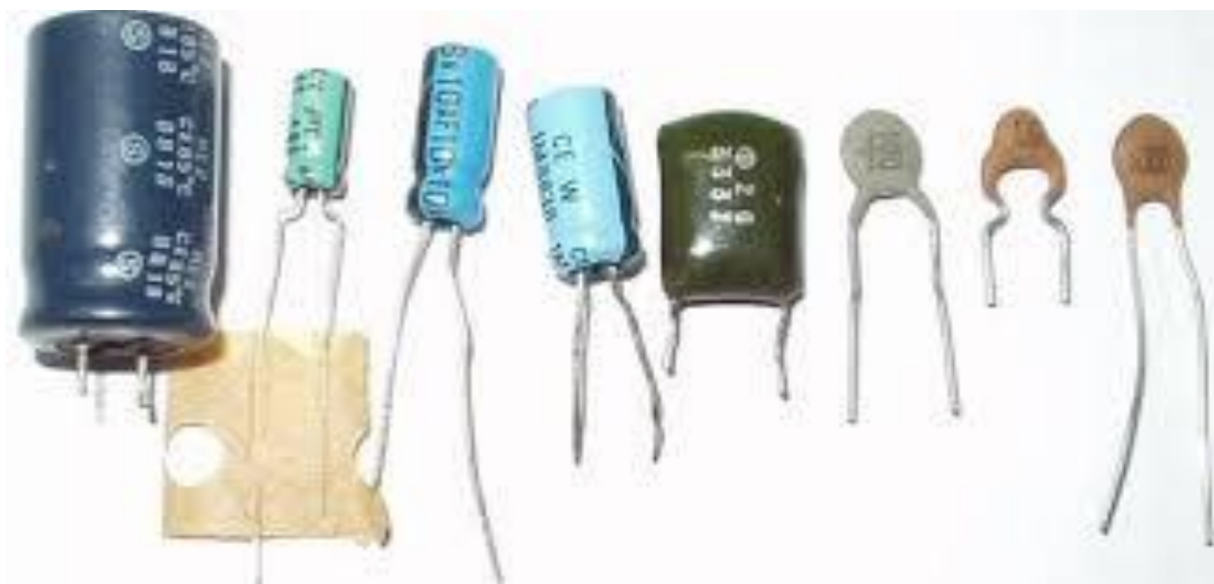
Figure (15): Fixed Capacitors
