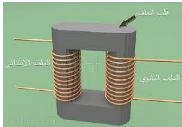
Figure (18): An inductor with a magnetic core
