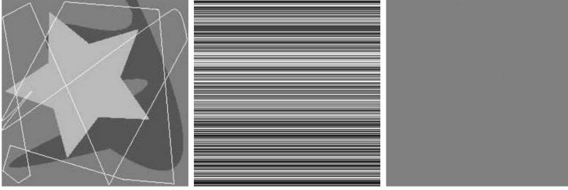
Figure 3.1: Computer generated 256 \times 256 \times 8 bit images with (a) coding redundancy, (b) spatial redundancy, and (c) irrelevant information. (Each was designed to demonstrate one principal redundancy but may exhibit others as well.)
