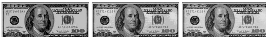
Figure 2.14: Images reconstructed using (a) bit planes 8 and 7; (b) bit planes 8, 7, and 6; and (c) bit planes 8, 7, 6, and 5. Compare (c) with Fig. 2.13(a).
