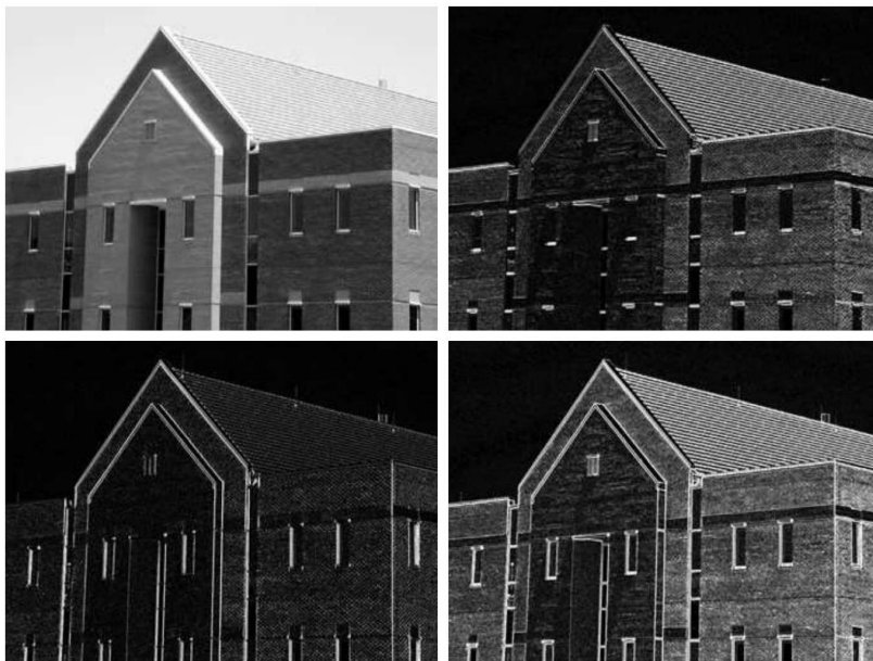
Figure 4.14: (a) Original image of size 834 \times 1114 pixels, with intensity values scaled to the range [0, 1] . (b) |g_x| , the component of the gradient in the x -direction, obtained using the Sobel mask in Fig. 4.12(f) to filter the image. (c) |g_y| , obtained using the mask in Fig. 4.12(g). (d) The gradient image, |g_x| + |g_y| .
