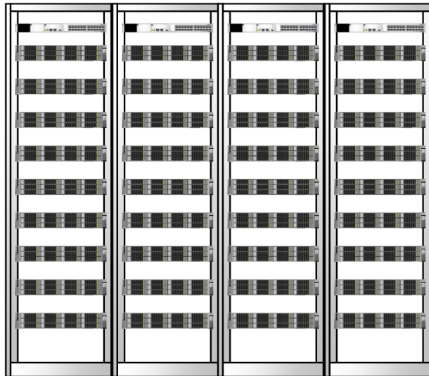
Figure 3-6 ToR cabling mode
