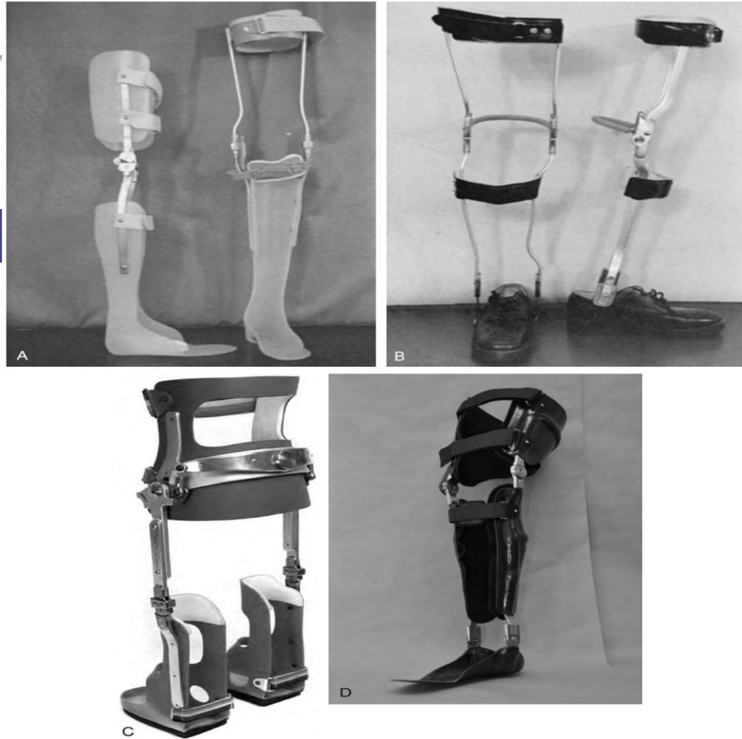
Fig. 13.18 A , Combination plastic and metal knee-ankle-foot orthoses. B , The Scott-Craig knee-ankle-foot orthosis is a special design for spinal cord injury. The orthosis consists of double uprights, offset knee joints with locks and bail control, one posterior thigh band, a hinged anterior tibial band, an ankle joint with anterior and posterior adjustable pin stops, a cushion heel, and specially designed footplates made of steel. C , The reciprocating gait orthosis, although generally used with children, is also used with adults. Its main components are a molded pelvic band, thoracic extensions, bilateral hip and knee joints, polypropylene posterior thigh shells, ankle-foot orthosis sections, and cables connecting the two hip joint mechanisms. D , Electronic knee-ankle-foot orthosis. ( A–C , From Umphred DA, editor: Umphred's neurological rehabilitation , ed 6, St. Louis, 2013, Elsevier; D , From Webster JB, Murphy DP, editors: Atlas of orthoses and assistive devices , ed 5, St. Louis, 2019, Elsevier, p 253.)
