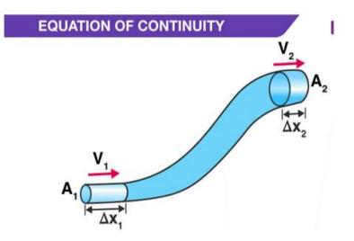
Now, consider the fluid flows for a short interval of time in the tube. So, assume that short interval of time as  $\Delta t$ . In this time, the fluid will cover a distance of  $\Delta x_1$  with a velocity  $v_1$  at the lower end of the pipe.
