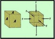
a bulk modulus B of elasticity.
