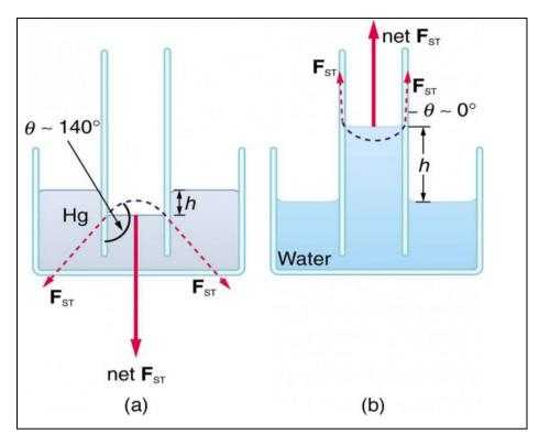
A simple relationship determines how far the water is pulled up the tube (see Figure 5). The force upwards due to the surface tension is given by the following relationship:  $F_{up} = \gamma (2\pi a) \cos \theta$
