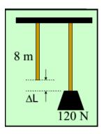
$Y = 8.96 \text{ x } 10^{11} \text{ Pa; } F = 120 \text{ N; } L = 8 \text{ m; } A = 1.77 \text{ x } 10^{-6} \text{ m}^2 \text{; } F = 120 \text{ N; } \Delta L = ???$
