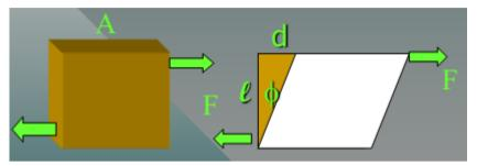
The shearing force F produces a shearing angle  $\phi$ . The angle  $\phi$  is the strain and the stress is given by F/A as before.
