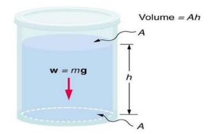
Pressure is the weight of the fluid *mg* divided by the area *A* supporting it (the area of the bottom of the
