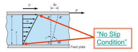
We feel resistance if we walk into a lake. This means the existence of a force of friction in water. It is notable that this force differs from a liquid to another; there are liquids of high friction force and others of low friction force. Forces of friction of these liquids are known as viscosity of liquids or fluids. If the force is high the liquid or fluid is said to be highly viscous and vice versa.
