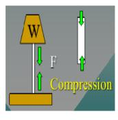
Strain is the relative change in the dimensions or shape of a body as the result of an applied stress:
