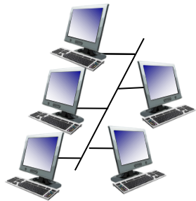
shared wire (e.g., cabled Ethernet)
